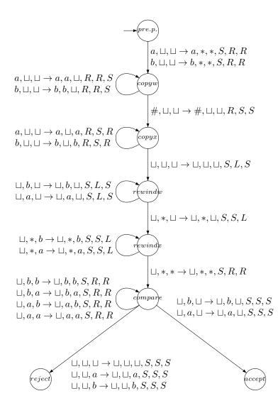
For this TM, I am using three tapes, the first for the input w # x, in the second I make a copy of w and in the third a copy of x. I am using the letter S in addition to L and R to indicate that the header should stay in the same place for a given tape.
